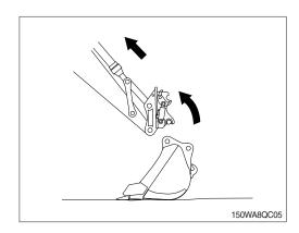
(9) To lock the quick coupler, release the quick coupler button on the right RCV lever.
